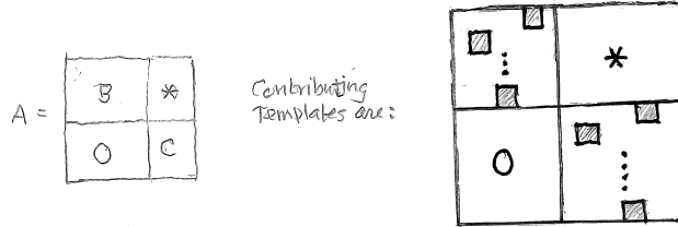
Figure 5.2. If A is a block upper-triangular square matrix, then \det(A) = \det(B) \cdot \det(C) and the only templates that contribute to \det(A) are those whose marked spots lie entirely within the blocks B and C .
